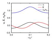
NB: electric field and density 90° out of phase
