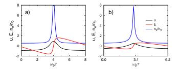
Typical features : i) sawtooth electric field; ii) spiked density; iii) *lengthening* of the oscillation period by factor  $\gamma$ .
