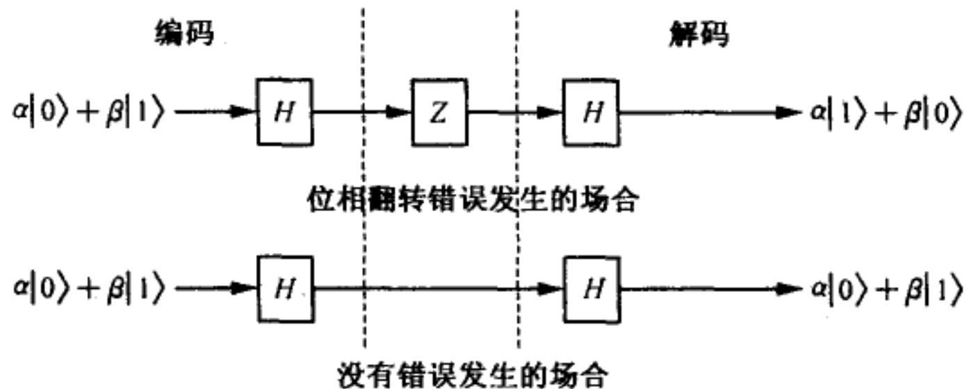
$$|+\rangle = H|0\rangle = \frac{1}{\sqrt{2}} \begin{bmatrix} 1 & 1 \\ 1 & -1 \end{bmatrix} \begin{bmatrix} 1 \\ 0 \end{bmatrix} = \frac{1}{\sqrt{2}} \begin{bmatrix} 1 \\ 1 \end{bmatrix}$$
